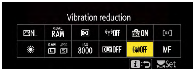
Figure 3.5: The stabilizer must also be switched off, preferably in the camera and also at the lens (if present).
